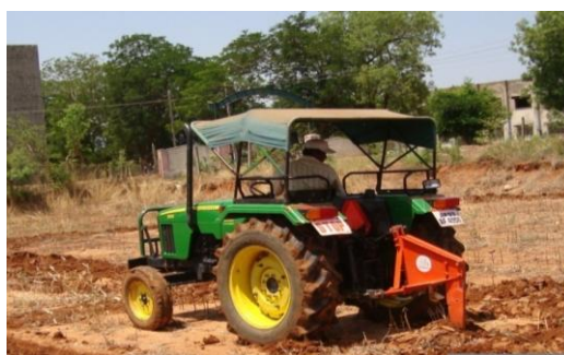
Sub soiler (up to 70 cm) for better moisture retention
